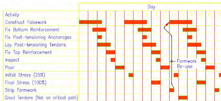
Figure 4. Typical 5 day construction cycle. Note that in tower construction it is usual to break the floor into a minimum of two pours. The above cycle is for a half floor with construction of the other half proceeding simultaneously.
