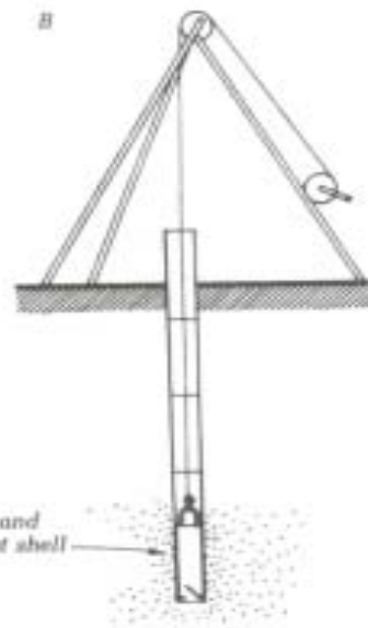
Sinking tubes through ballast
